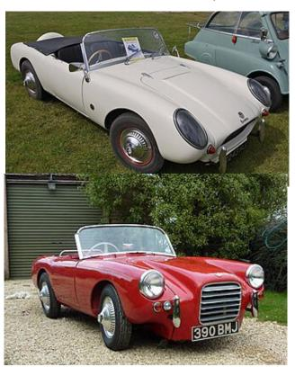
Berkeley Foursome. 1958–1959. 20 approx produced. 492 cc transverse two stroke three cylinder, air-cooled. Note cover over tiny rear seats behind cockpit and spare wheel, now mounted over rear bumper. The body was somewhat wider and longer and the suspension was revised to accommodate.
