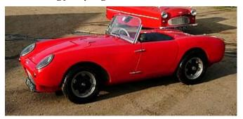
Berkeley Sports SA 322. Oct '56 – Jan '57. 163 produced. Anzani 322 cc transverse twin engine, aircooled. Curb weight 605 lbs. Three speed gear change on the steering column.
