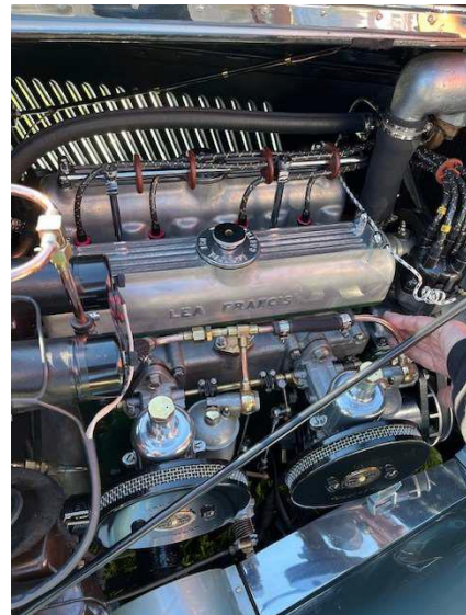
Here is an interesting British car I had never seen in person before: a Lea Francis. This is a 1940 Corsica model. The engine is interesting with its “cam in head” design. The camshafts are mounted just below the valves making for short and therefore stout, pushrods. Most other pushrod engines of the time were long stroke engines with the cams mounted low making for long, flexible, and fragile pushrods.
