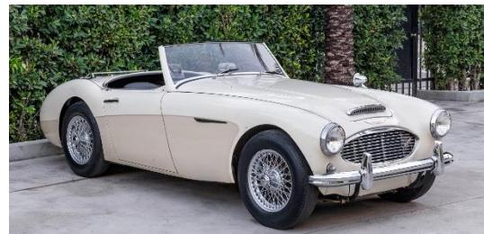
**3000 Mk II** 1961-1962. Mk II badging. Only 355 two-seaters vs. 5,095 2+2 built! Triple SU carbs, (132bhp) abandoned the following year. Specs show it to be two mph slower than the two-carb MKI, and 2 mpg less! Still called the BN7 and BT7. A new gearbox in 1961 with improved remote shift linkage. Keeping the engine in tune led to abandoning the triple-carbs.
