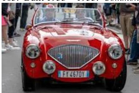
**100S:** 1955, 50 cars built at Healey's factory in Warwick. Light weight version of the BN1. Oval grill, no bumpers. Four speed manual transmission w/o overdrive. Max speed 117 mph. Four-wheel disc brakes.
