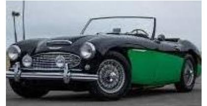
**3000 Mk I BN7** 1959-1961. Near identical with 100-6 except for badging. The engine was enlarged to 2.9 liters (124bhp vs. 117), more suitable gear ratios in the tranny. Most with wire wheels and overdrive and 2+2 seating (hilarious for a guy who was 6'4" from 17 to age 70). The "four-seat models were designated **BT7**. Front disc brakes. Max speed 114mph. Assembled in the Abington factory, which was an assembly facility only, not a manufacturing factory!
